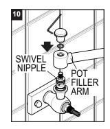
Loosen the Set Screw in the Tie Down Cap and remove the Cap. Then remove the **small** Teflon Washer only. Leave the larger Washer on top of the Swivel Nipple.
