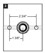
Rough-In plumbing should ensure that the 1/2" NPT Nipple (not supplied) protrude not less than 3/4" and not more than 1" from the Finished Wall.
