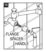
Screw the Flange onto the Cartridge as far as it will go, then fit the Teflon Spacer into the Flange as shown. Make sure the Cartridge is in the **OFF** position and assemble the Handle accordingly and secure by tightening the Set Screw with the Allen Key provided.
