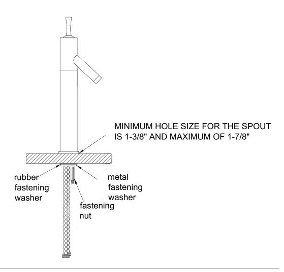
\*\*\* NOTE: SHUT OFF WATER SUPPLY BEFORE BEGINNING INSTALLATION\*\*\*
