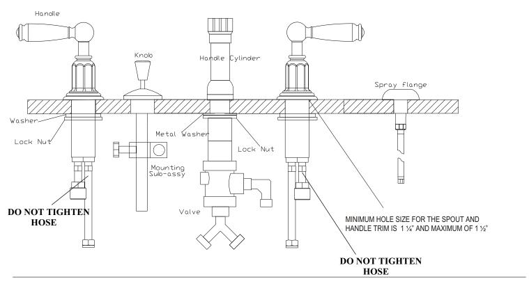
\*\*\* NOTE: SHUT OFF WATER SUPPLY BEFORE BEGINNING INSTALLATION\*\*\*
