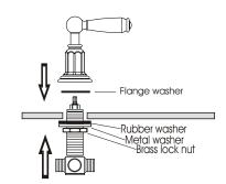
\*\* The spout, handle valve bodies and diverter can be connected with flex hoses (not provided by Santec) or copper pipe soldering. Please note that when soldering connections, do not use excessive heat. Excessive heat can damage the joints increasing probability of leakage.
