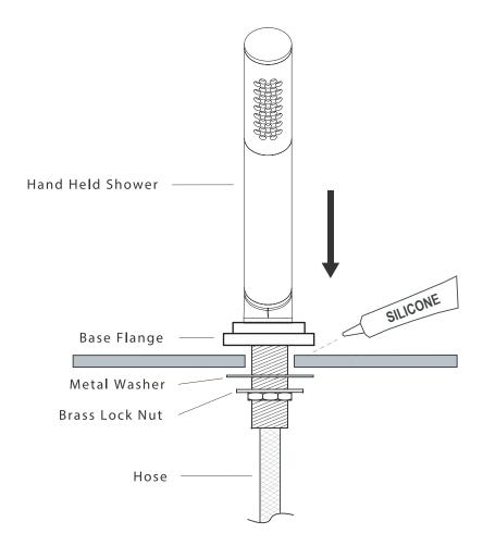
Other end of Hose to connect to Spout Diverter Valve
