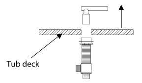
3 -Slip valve body up from below tub deck.
