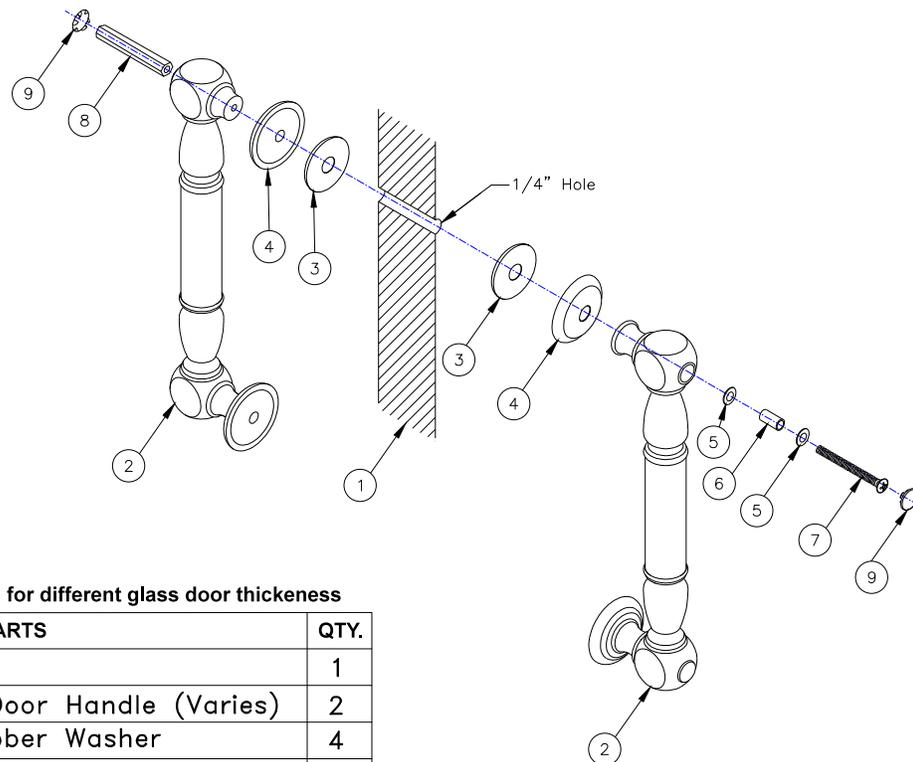
\*Screw is able to be cut in field for different glass door thickness
