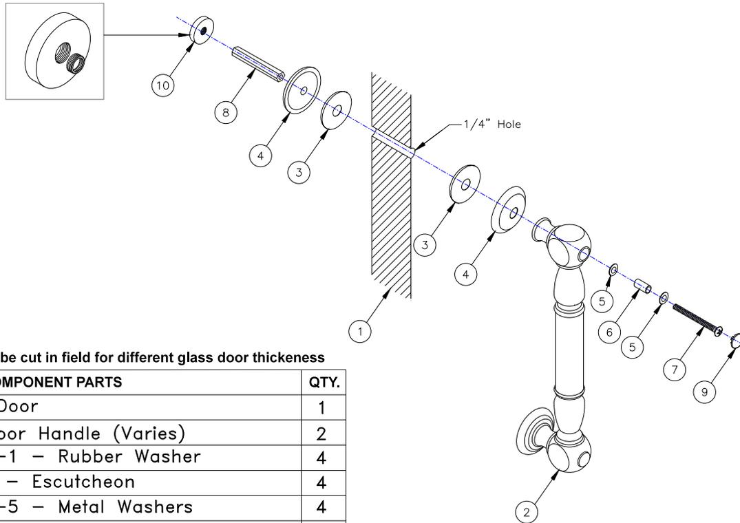
\*Screw is able to be cut in field for different glass door thickness
