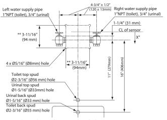
X", ‡ = At least 5" clearance from sensor to tip of toilet seat up position or to top of grab bar is required to avoid false detection.
