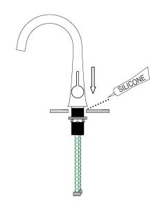
Reinstall rubber washer and metal washer from below. Hand tighten lock nut from below while aligning fixture.
