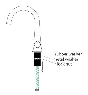
Apply a ring of silicone caulking around hole designated for spout. DO NOT USE PLUMBERS' PUTTY WHICH CAN DAMAGE FINISH. Insert faucet assembly through hole in sink or counter top, being sure to center faucet in hole.
