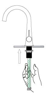
4 Secure fixture below by using either an adjustable wrench, basin wrench, or deep socket to the lock nut. Wipe away excess silicone with a wet finger or damp cloth. Connect flexible hoses to their respective water supplies.
