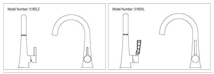
Flush both supply lines before installation, then shut off both supply lines. Minimum hole size for the spout and handle trim is 1-1/4" and maximum of 1-1/2"
