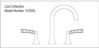
Flush both supply lines before installation, then shut off both supply lines. Minimum hole size for the spout and handle trim is 1-1/4" and maximum of 1-1/2"
