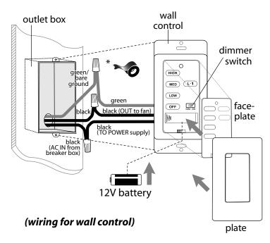
\* Wrap each wire connector separately with electrical tape as an extra safety measure.
