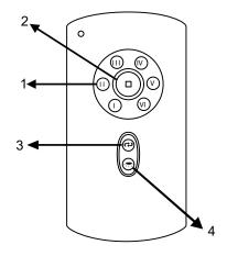
Fan **SPEED** buttons--1: Fan **OFF** button--2: **REVERSE** function button--3: **LIGHTING** button--4: Use to control ceiling fan speeds 1-6 Use to turn the fan off Use to control fan direction Use to control down-light and up-light (not applicable for this fan)
