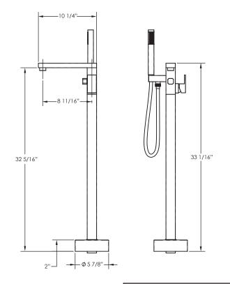
Ensure that the supply lines protruding from finished floor is in the MIN-MAX area
