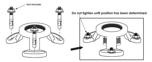
Connect Supply Hoses to lines on floor. Then attach the Tub Filler to the mounting base, followed by sliding down the cover base.
