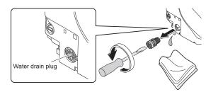
Reinstall the water drain plug and cover.
