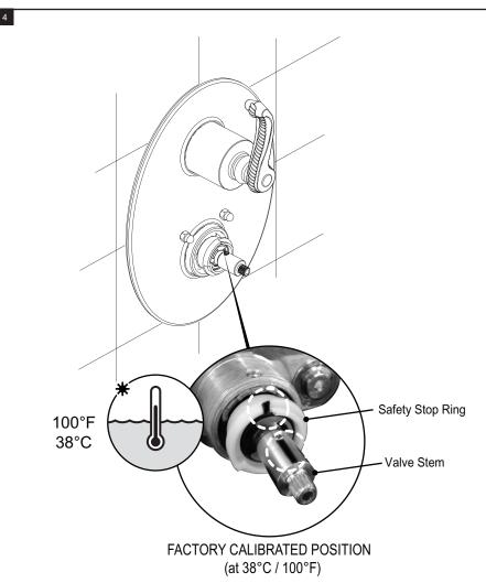
Before installing the Handle make sure that the red marks on the valve stem and safety stop ring are at 12 o'clock position as shown above. It corresponds to approximately 100 F (38 C) temperature of the discharging water.
