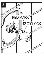
Remove the Screw and Lock Washer and Spline from the Handle assembly.
