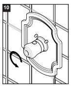
Turn the Handle clockwise and then counter clockwise until it stops. The Handle should now be in the 12 o'clock position and the Valve should discharge water at approximately 100°F (38°C).
