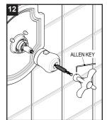
With the Handle removed turn the Valve Stem clockwise or counter clockwise using pliers to adjust the temperature either up or down until the temperature of 100°F (38°C )is reached.
