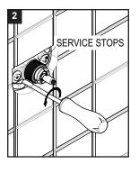
Remove the Mounting Jig and Sleeve only when tiling is complete. Check that both Service Stops are open using a 3/16" flat screwdriver and turning the stems counter clockwise until they stop.
