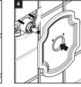
Insert the Threaded Rods in the Thermostatic Valve and thread the Valve Sleeve onto the Valve as shown.
