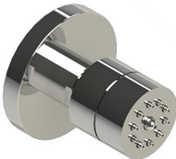
BODY SPRAY WITH 1/2" NPT X 1/2" NPSM X 3" NIPPLE X QTY 4 INCLUDED
