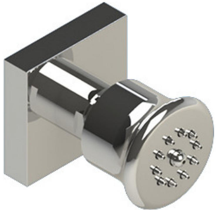
BODY SPRAY WITH 1/2" NPT X 1/2" NPSM X 3" NIPPLE X QTY 4 INCLUDED
