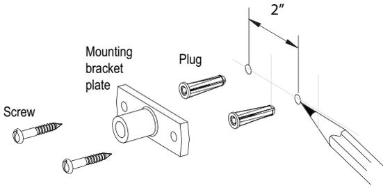
MARK ANCHOR HOLES FOR MOUNTING BRACKETS. THEN DRILL  $\varnothing$  1/4" HOLES FOR ANCHORS.
