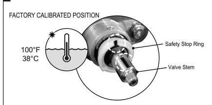
Before installing the Handle make sure that the red marks on the valve stem and safety stop ring are at 12 o'clock position as shown above. It corresponds to approximately 100 F (38 C) temperature of the discharging water.
