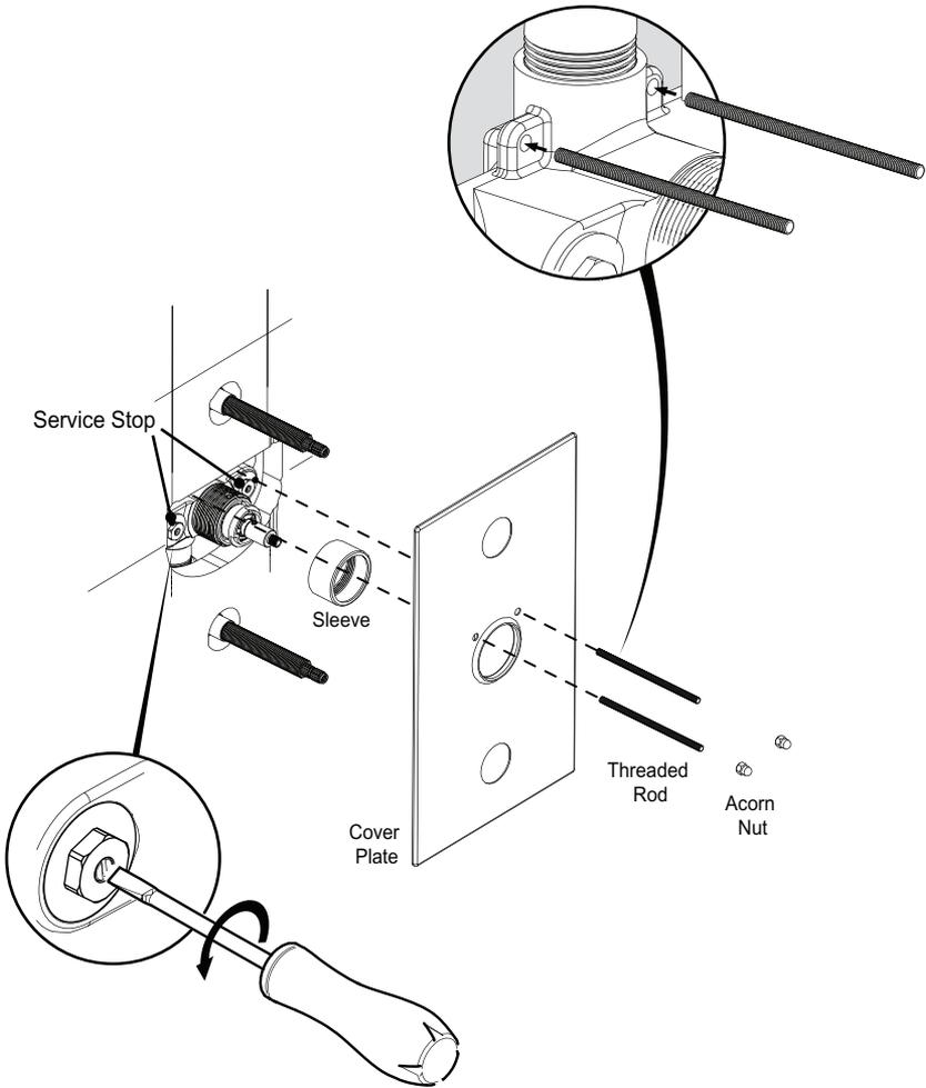
Check both Service Stops are open using a 3/16" flat screwdriver and turning the stems counter clockwise until they stop.
