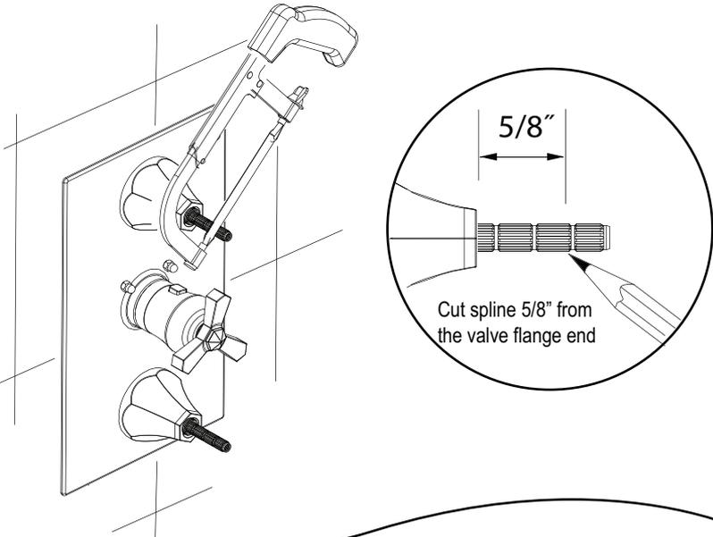
Turn cartridge spline into OFF position before installing handles
