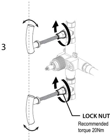
Turn the handle towards the desired ON alignment. Then tighten the lock nut to secure. This adjustment should not be more than 25°.
