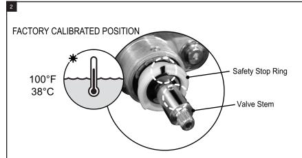
Before installing the Handle make sure that the red marks on the valve stem and safety stop ring are at 12 o'clock position as shown above. It corresponds to approximately 100 F (38 C) temperature of the discharging water.
