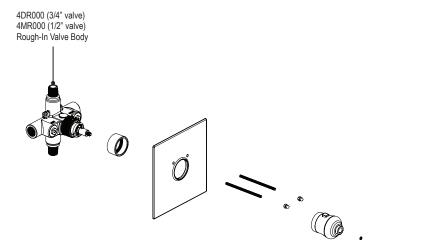
TEMPERATURE CONTROL VALVE WITH BUILT-IN STOPS
