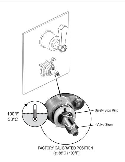
Before installing the Handle make sure that the red marks on the valve stem and safety stop ring are at 12 o'clock position as shown above. It corresponds to approximately 100 F (38 C) temperature of the discharging water.
