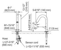
■Mounting deck thickness: 1/4" (5 mm) - 2" (50 mm) ■Spout hole: Ø1-1/4" (Ø32 mm) - Ø1-3/8" (Ø35 mm)
