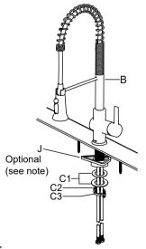
Install the plastic washer and metal washer (C1) onto the threaded mounting shank. Thread the nut (C2) onto the mounting shank. Lock the nut (C2) into position by tightening the screws (C3). Do not overtighten.
