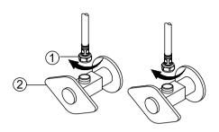
Thread the nut (1) on the supply line onto the outlet of the water supply valve (2) and tighten with wrench. Do not overtighten.
