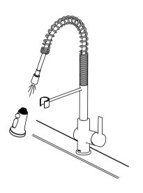
Pull hose assembly out of spout and remove spray head by unscrewing from hose in a counterclockwise direction. Hold the end of the hose down into the sink and turn the faucet on to the warm position. Flush water lines for one minute to flush away any debris. Check for leaks.
