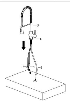
Before installation, ensure that the flange (D) is placed on the bottom of the new faucet assembly (B). Insert the faucet body and all hoses through the hole in the sink.
