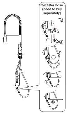
Connect the 3/8 in. water line from the filtration system by pushing the line into the connector (G). Pull down on the 3/8 in. line slightly to ensure the quick connect fitting has engaged.
