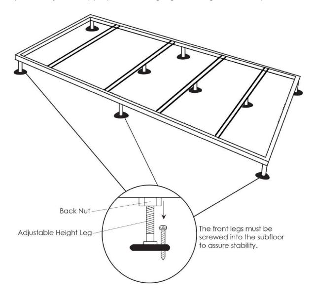
Layout of adjustable leveling legs varies by model. This may not be an exact representation of how your tubs leveling legs are laid out. This is to be used as an example and to show that the legs need to be secured to the sub-floor.
