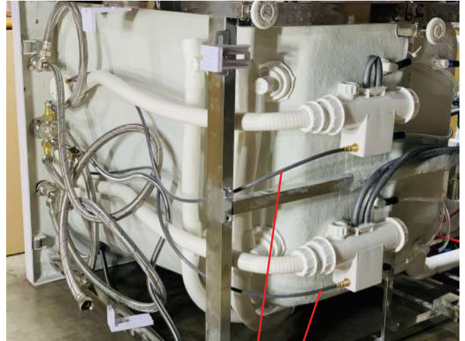
Stainless steel drain operating cable
