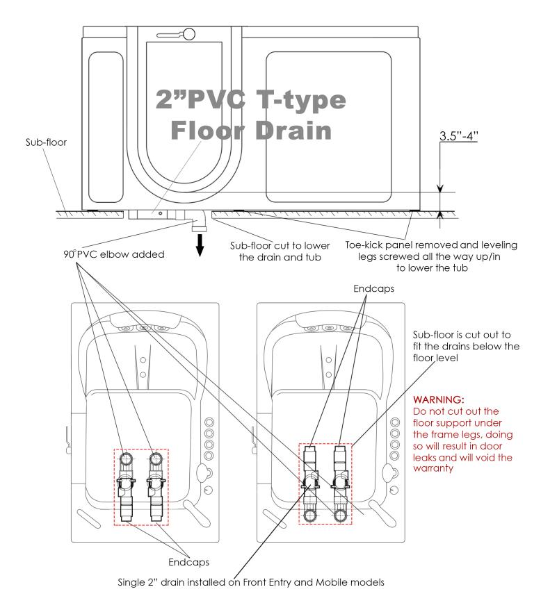
The drain positioning should be determined by a licensed plumber. The pictures above only show a few of the many possible options for drainage setup. For faster drainage all 4 ports may be connected to house drain.
