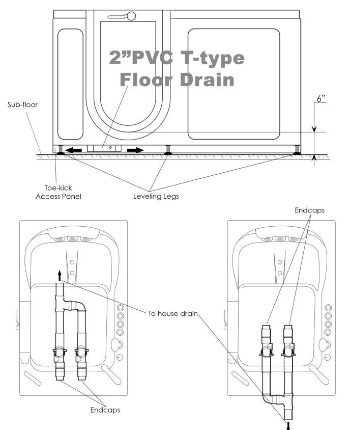
The drain positioning should be determined by a licensed plumber. The pictures above only show a few of the many possible options for drainage setup. For faster drainage all 4 ports may be connected to house drain.
