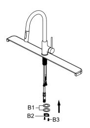
Install the rubber washer and metal washer (B1) onto the threaded mounting shank. Thread the nut (B2) onto the mounting shank. Lock the nut (B2) into position by tightening the screws (B3). Do not overtighten.
