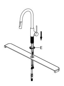
Insert all the hoses through the Base Seat Assembly (E). Insert the faucet body through the hole in the sink or countertop.
