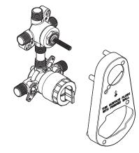
M-CORE™ With Integrated 2 Function / 3 Function Transfer Valve
