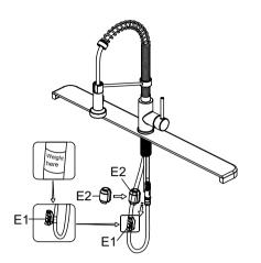
Install the weight clip (E1) at the point of the hose marking "weight here". Insert the weight (E2) onto the clip (E1) by sliding it down onto the clip (E1).
