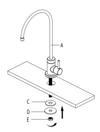
Place the faucet assembly (A) through the selected hole in the sink or countertop. On the underside of the sink or countertop, slide the rubber washer (C) and metal washer (D) onto the stud. Thread the mounting nut (E) onto the stud, and tighten securely using your wrench.
