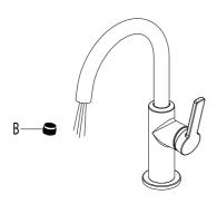
After installing the faucet, remove the aerator (B) with a coin. Turn the water on for 30 seconds to remove any debris. Reassemble the aerator (B).
