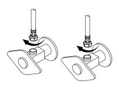
Attach waterlines to angle stops and tighten until snug. Turn on angle stops and check for leaks (DO NOT TURN FAUCET ON).
