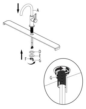
Place the faucet (A) through the hole in the sink or countertop. Secure the faucet (A) to the countertop using the plastic washer (D), metal washer (E) and mounting nut (F) provided. Tighten screws (G). Do not overtighten.
