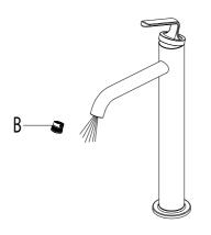
After installing faucet, remove aerator (B) with a coin. Turn water on for 30 seconds to remove any debris. Reassemble aerator (B).
