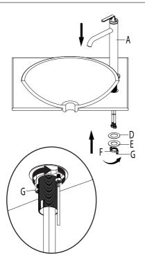
Place the faucet (A) through the hole in the countertop. Secure the faucet (A) to the countertop using the plastic washer (D), metal washer (E) and mounting nut (F) provided. Tighten screws (G).
