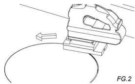
2. Cut out the counter -The cutting tools required will depend on the surface to be cut. FG.2 (Your sink comes with 4 mounting screws for mechanical fastening. Screws are only necessary if for some reason silicone cannot be used. In this case, you will need to drill 4 holes in the counter to accommodate these screws)
