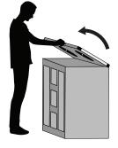
Lower the counter so that it lays flat on the cabinet, while supporting it from the side and front. Be careful not to catch your fingers under the counter. It is best to lower the counter by supporting from the front as it comes down onto the cabinet.
