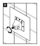
With the Override Button at 12 o'clock and lined up with the Red Mark on the Valve Stem install the Handle.
