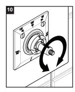
To test the water temperature turn on one of the Volume Control Shut-Off valves down stream from the Thermostatic Valve.
