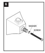
Before installing the Handle make sure the Red Mark on the Valve Stem lines up with the Red Mark on the Stop Ring in the 12 o'clock position.
