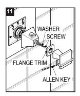
With the temperature set replace and assemble the Handle as shown.
