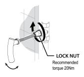
Turn the handle towards the desired ON alignment. Then tighten the lock nut to secure. This adjustment should not be more than 25°.
