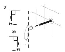
Replace handle one tooth off from the OFF position as shown (try both direction as needed)
