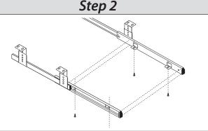
Align the shelf 1/16" shorter than the slide plastic protector. Fasten shelf with (4) recommended #8 x 5/8" pan head wood screws
