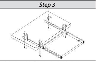
With the drawer slides fully closed, mark the bracket locations so shelf is 1/4" - 1/2" shorter than the front edge of the table. Fasten shelf with (8) recommended #8 x 5/8" pan head wood screws
