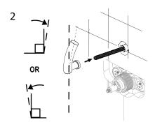
Replace handle one tooth off from the OFF position as shown (try both direction as needed)
