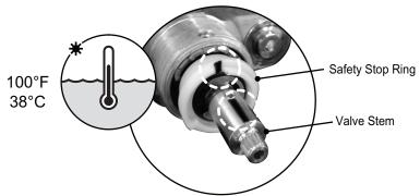
Before installing the Handle make sure that the red marks on the valve stem and safety stop ring are at 12 o'clock position as shown above. It corresponds to approximately 100 F (38 C) temperature of the discharging water.
