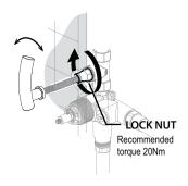
Turn the handle towards the desired ON alignment. Then tighten the lock nut to secure. This adjustment should not be more than 25°.
