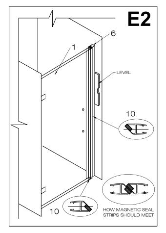
3. Mark the wall on both sides of the vertical track (#6). The vertical track should be installed with the bottom resting on the floor
