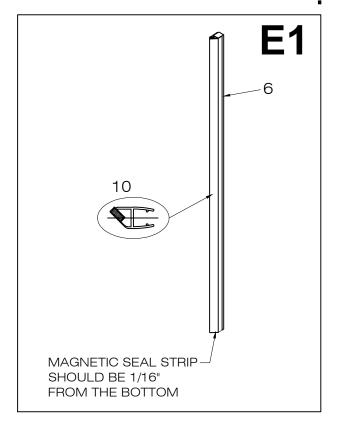
2. Attach the door magnetic seal strips (#10) to each other and then close the door, making sure the door is on a level plain, keeping the walls and opening at a perfect 90° angle.
