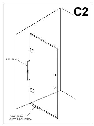
3. Hold the door in the open position and mark two (2) holes on the wall for the mounting screws for each hinge.
