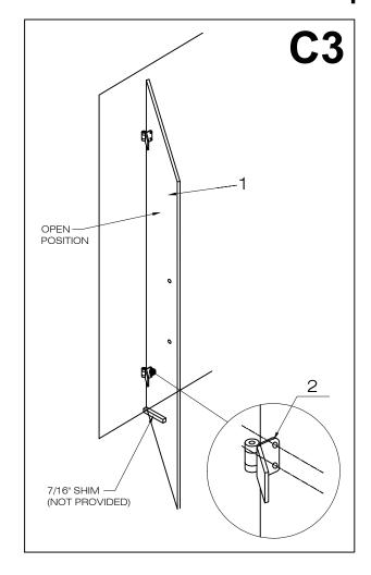
4. Remove the door and drill holes into the wall where marked. Place plastic anchors (#8) inside the holes. Not necessary if installing into studs. Studs are the preferred means of installation, anchors can pull out of the wall causing property damage and bodily harm.
