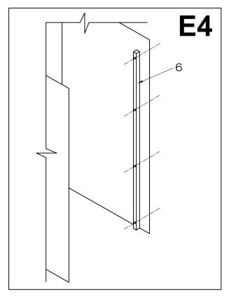
5. Remove the vertical track, pre-drill and sink plastic anchors (#11) into the wall. Not necessary if installing into studs. Studs are the preferred means of installation, anchors can pull out of the wall causing property damage and bodily harm.
