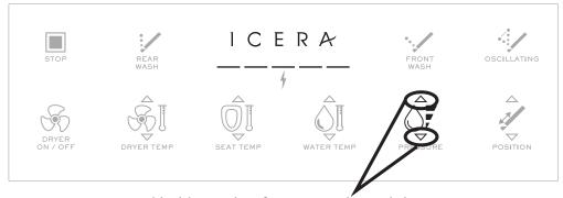
**FIRST:** Press and hold together for 4 seconds until the channel indicator light turns on.
