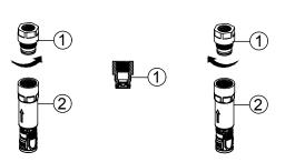
This faucet ships with a 1.8 GPM flow restrictor installed. An optional 2.2 GPM flow restrictor is also included in the box.
