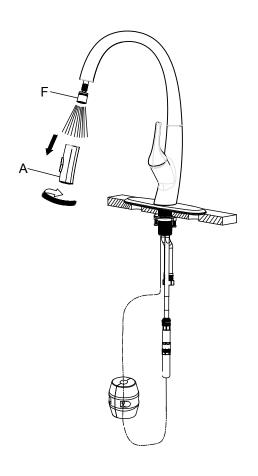
Remove spray head (A). Hold tip of spray hose (F). Turn faucet on for 1 minute to flush any debris.
