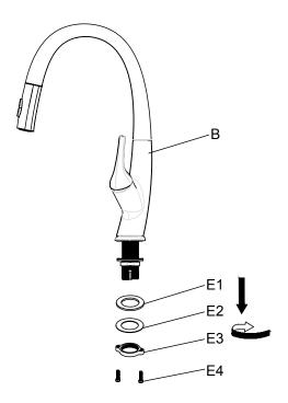
Shut off the water supply. Remove the old faucet. Clean the mounting surface. Remove mounting hardware (E) from faucet body (B).
