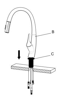
For single-hole installation, deck plate assembly (D) and silicone sealant are NOT required.
