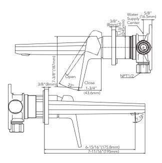
NOTE: Unit for dimensions = inches Dimension in ( ) is mm.
