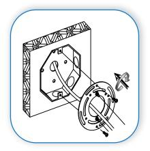
If there is an existing fixture remove it. Expose the supply wires from the J-box. Install the crossbar plate and mount it to the J-Box
