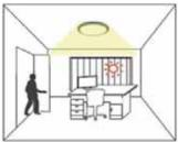
The fixture will turn on when motion is deteted, regardless of the presense of natural light.
