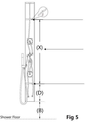
Mark bottom position of upper metal support on wall. Add **(B)+(D)+(X)**= Distance from floor to bottom of top metal support
