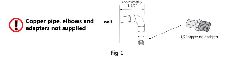
**2.** Using a helper, place the unit against the shower wall at the desired position (over the two stub-outs) with the showerhead about 12"-18" above average head height **(A)**. Plumb the unit with a level and mark the wall on the side of the unit as well as at the bottom of the unit. Remove the unit from the wall and carefully put it aside. **(B)** Represents the distance from the floor to the bottom of the unit. **(Fig 2)**
