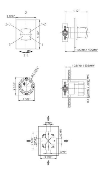
Lady ¾" thermostatic valve only ¾" inlet connections Rough included.
