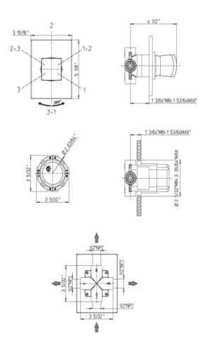
Lady 3-way diverter 3/4" ceramic disk valve 1/2" inlet connections Rough included.
