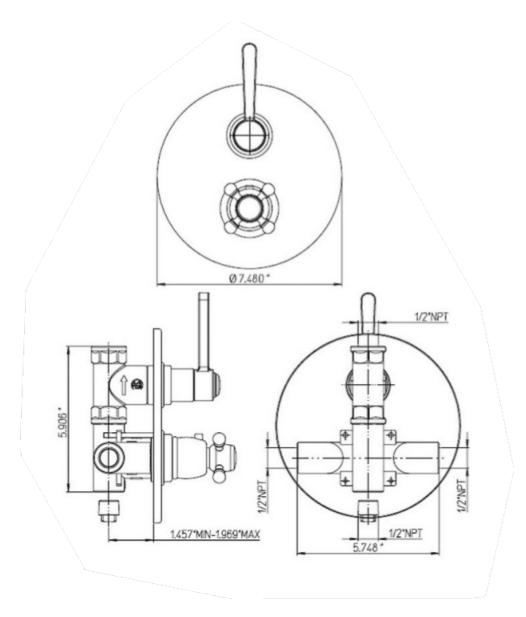
Firenze thermostatic valve with <sup>3</sup>⁄<sub>4</sub>" ceramic disk volume control <sup>1</sup>⁄<sub>2</sub>" inlet connections
