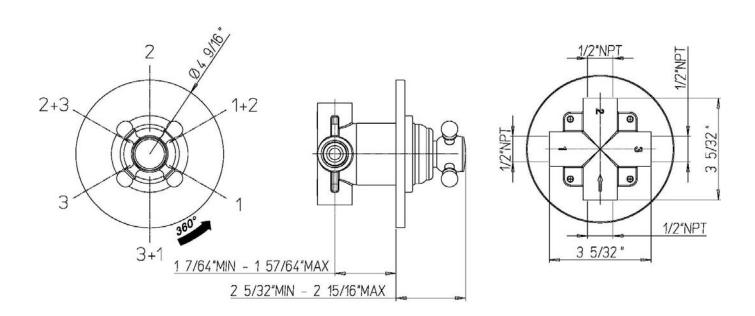
Firenze 3-way diverter <sup>3</sup>⁄<sub>4</sub>" ceramic disk valve <sup>1</sup>⁄<sub>2</sub>" inlet connections
